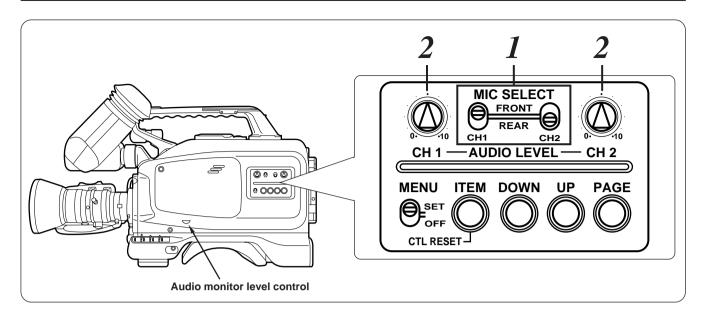
Select the desired input signals using the audio input selector switches.
